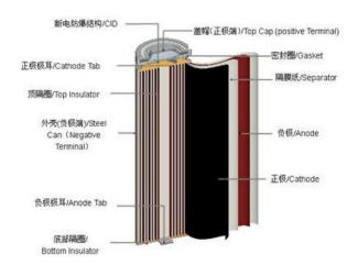
A cell is made of cathode, anode, separator, can and header.
